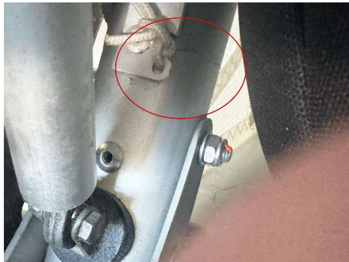
Figure B2 – Crack that will lead to failure
