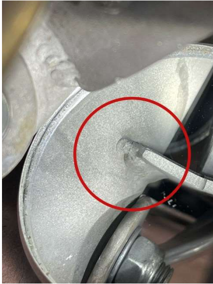
Figure C3 – visible crack on Bracket (Mirror view)
